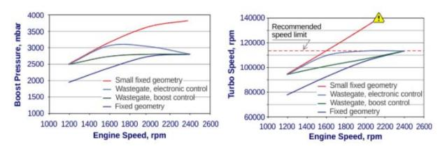
**Figure 23** Boost pressure and turbo speed for various types of turbochargers depending on engine speed [27]
