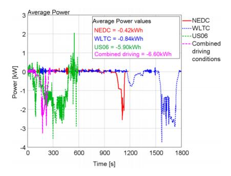
**Figure 43** Average power provided / harvested by the motor-generator where negative values indicate energy harvesting [45]
