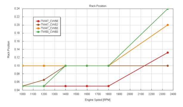
Figure 74 Rack position comparison
