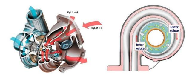
Figure 18 Twin scroll and dual volute turbine [26,13]
