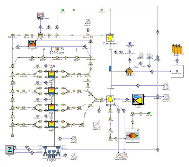
Figure 62 Engine model with motor-generator and battery
