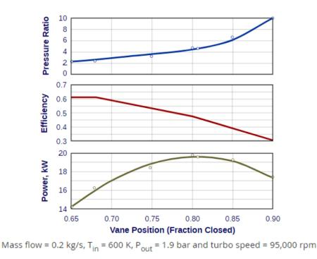
**Figure 34** Effect of turbine vane position on the turbine pressure ratio, efficiency and power produced by turbine for given conditions [28]
