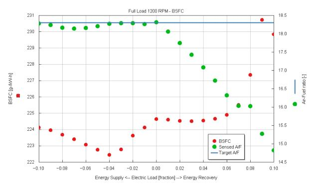
Figure 83 Electric load of E-Turbo affects BSFC
