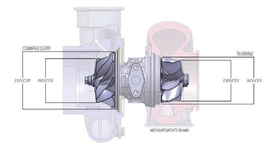
Figure 10 Exducer and inducer diameters of turbocharger [17]
