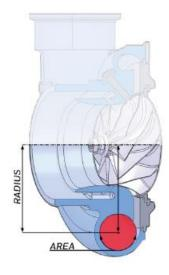
Figure 12 Area/Radius ratio of compressor housing [17]
