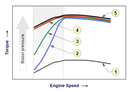
**Figure 45** Turbocharger assistance for improving low speed torque in downsized engines 1-Downsized engine, 2-Conventional turbocharger, 3-Variable geometry turbocharger, 4-VGT with motor assist, 5-Large displacement engine
