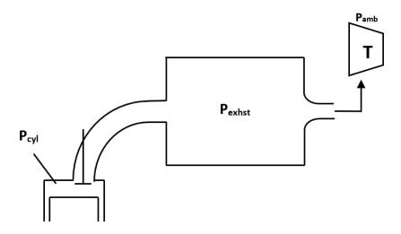
**Figure 5** Principle schematic diagram with constant-pressure tubocharging  $(P_{cyl}-cylinder\ pressure,\ P_{exhst}-exhaust\ pressure,\ T-turbine,\ P_{amb}-ambient\ pressure)$
