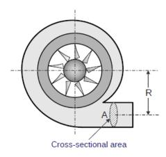
Figure 16 A/R ratio of turbine housing
