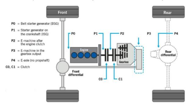
Figure 50 Position of electric motor in parallel hybrid architecture [54]
