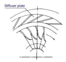
Figure 11 Radial compressor and vaned diffuser plate [13]
