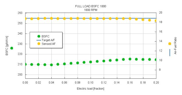
Figure 86 Electric load of E-Turbo affects BSFC
