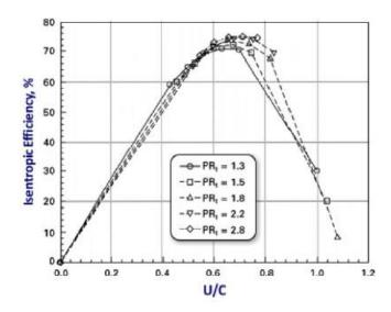
Figure 22 Turbine isentropic efficiency as function of blade speed ratio
