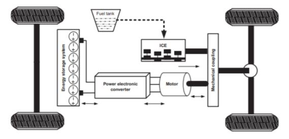
Figure 49 Architecture of parallel hybrid vehicle [52]
