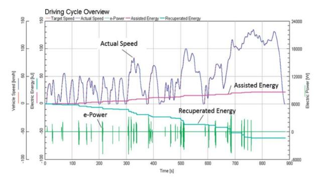
Figure 44 Kinetic energy recover from electrified tubocharger [46]
