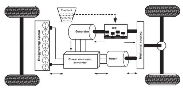
**Figure 51** Series-parallel architecture of hybrid vehicle [52]
