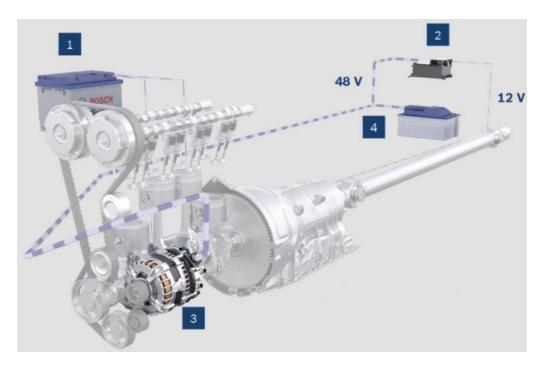
**Figure 53** Bosch 48V MHEV – components of the boost recuperation system 1 – low voltage battery (12V), 2 -DC/DC converter, 3 – electric motorgenerator, 4 – high voltage battery (48V) [55]
