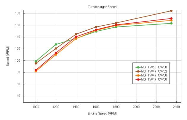
Figure 76 Turbocharger speed comparison
