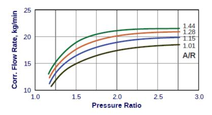
**Figure 17** Effect of A/R ratio on swallowing capacity (definition in subchapter 2.3.3) of an exhaust gas turbine [13]
