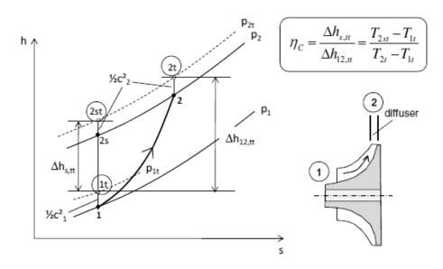
**Figure 37** Compression process in the compressor stage [1]
