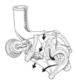
Figure 24 Gas flow though the turbine and wastegate [2]
