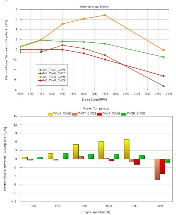
Figure 73 Energy recovery/supply comparison
