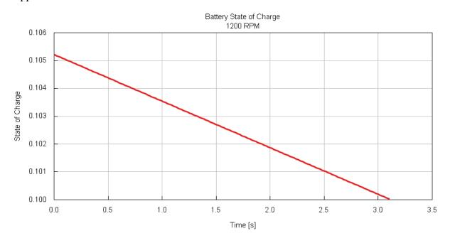
**Figure 85** Battery state of charge and supplying E-Turbo (discharging battery)
