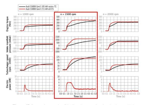
Figure 47 Comparison study of EAT and conventional turbocharger [41]
