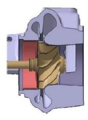
Figure 19 Asymmetrical twin scroll turbine [13]
