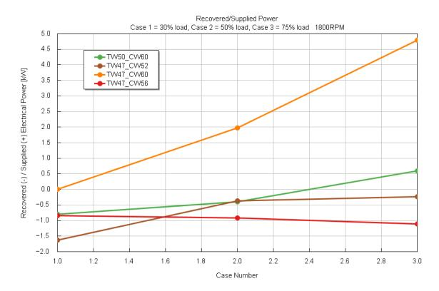
Figure 78 Energy recovery/supply comparison
