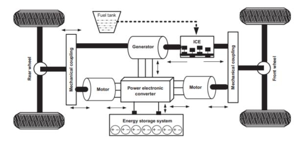
Figure 52 Architecture of complex hybrid vehicle [52]
