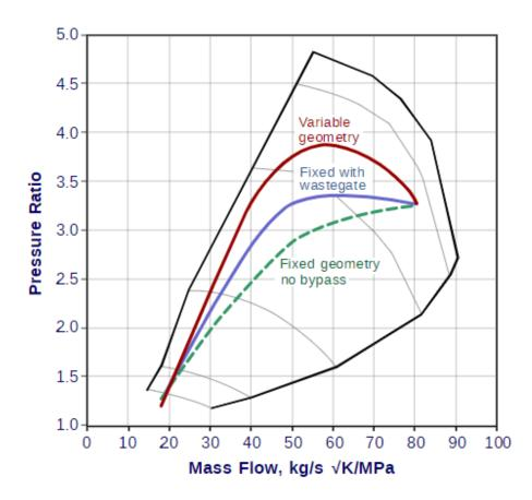
**Figure 32** Compressor map showing full load boost characteristics with three different turbine options [28]
