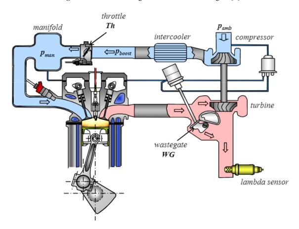
Figure 25 Wastegate turbocharger in spark ignition engine architecture
