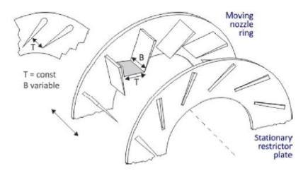
Figure 31 Moving nozzle or moving wall type variable geometry turbine [28]
