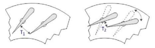
Figure 30 Pivoting vane variable geometry turbine [28]
