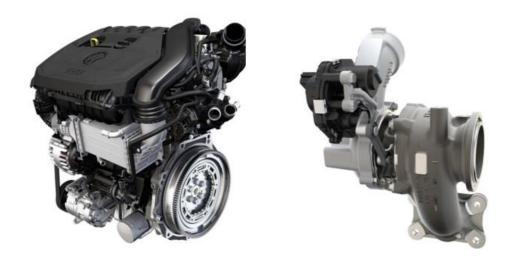
Figure 36 VW EA211 TSI evo and VNT turbocharger [31]
