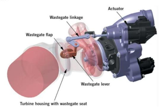
Figure 28 Wastegate turbocharger with electric actuator for BMW gasoline engine [30]
