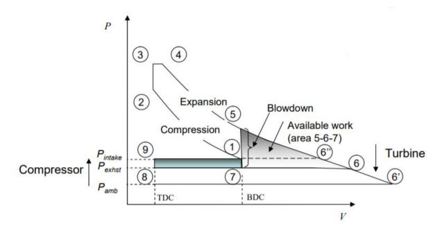
**Figure 4** Ideal P-V diagram of supercharged engine (P – pressure, V – volume,  $P_{intake}$  – intake pressure,  $P_{exhst}$  – exhaust pressure,  $P_{amb}$  – ambient pressure) [5]
