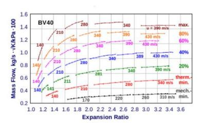
Figure 33 Variable vanes openings of VNT turbocharger in turbine characteristic
