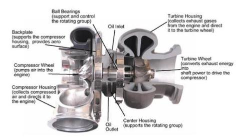
Figure 3 Section view of turbocharger [8]
