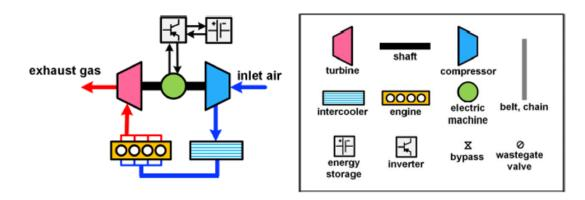
Figure 42 Schematic layout of engine with electrically assisted turbocharger [44]
