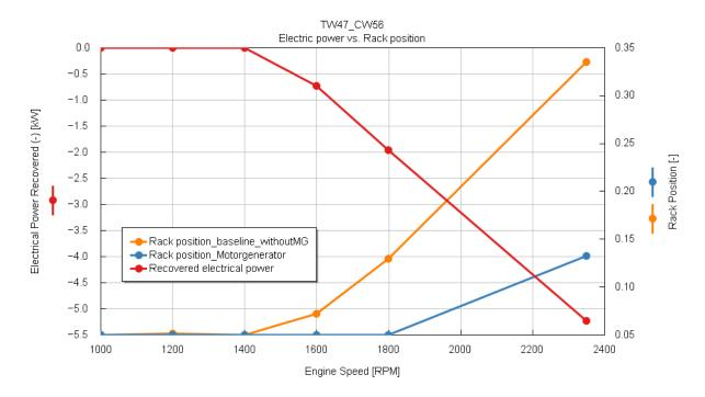
Figure 67 Differences in rack postion for engine models
