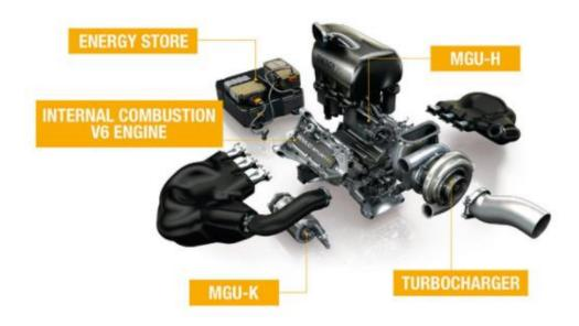
**Figure 41** F1 V6 hybrid powertrain with MGU-K and MGU-H generator units for energy recovering [43]
