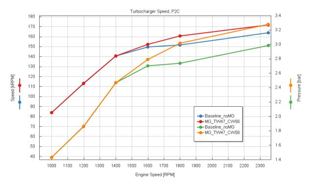
Figure 69 Turbocharger speed and post compressor pressure
