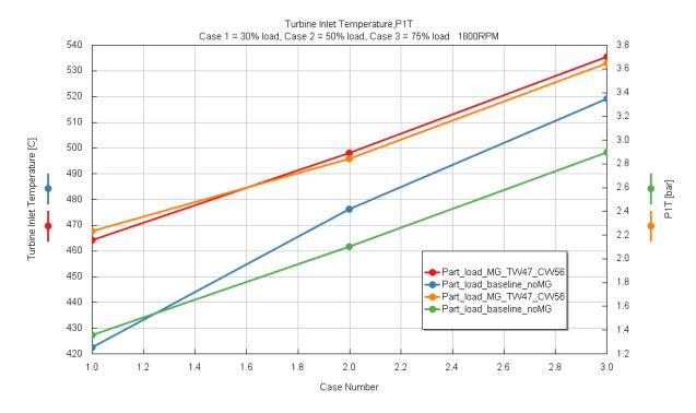
Figure 71 Part load comparison of turbine inlet pressure and temperature
