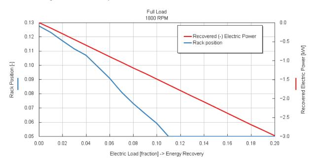
Figure 87 Energy and rack position comparison for specific electric load
