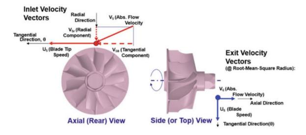
Figure 15 Velocity diagram of radial turbine [23]
