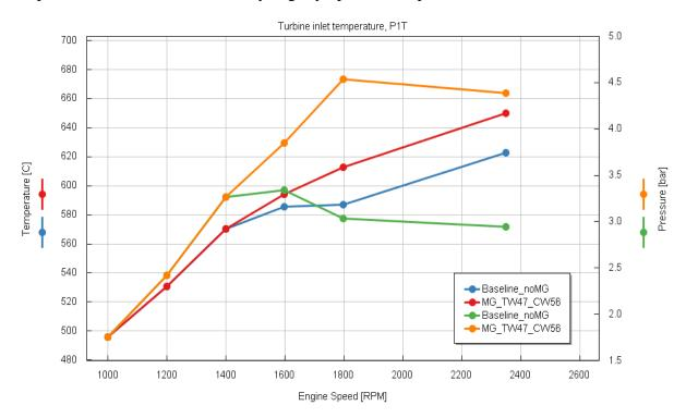
Figure 68 Pre-turbine pressure and temperature comparison
