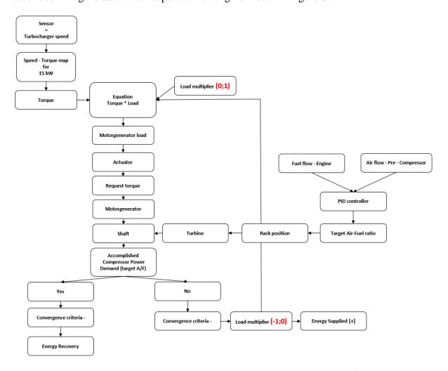
Figure 63 Flow chart map of controlling motor-generator load (2<sup>nd</sup> option)
