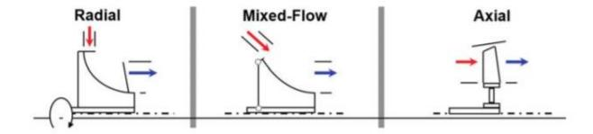
Figure 14 Types of turbines used in turbochargers [23]
