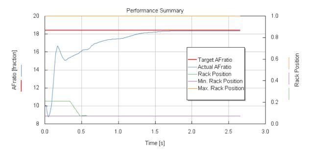
Figure 65 VNT controller for air-fuel ratio
