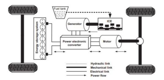
**Figure 48** Architecture of series hybrid vehicle [52]
