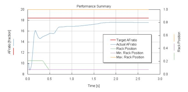
Figure 66 Too high E-turbo load
