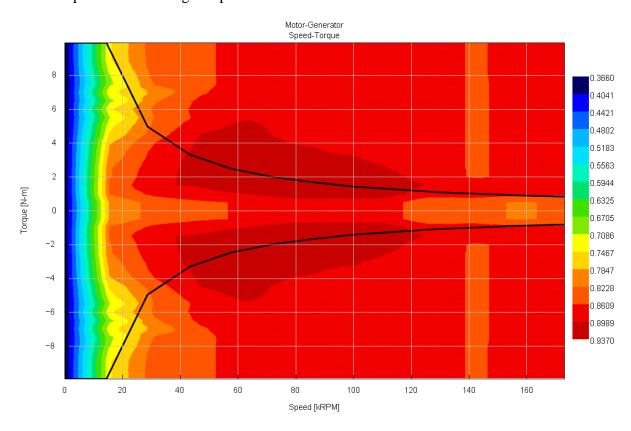
Figure 61 Motor-generator speed-torque efficiency map
