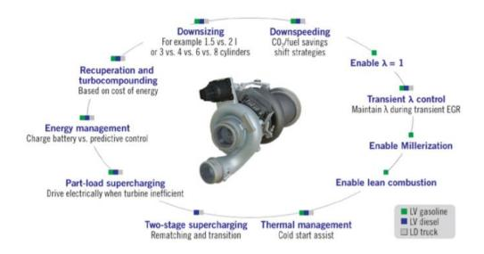
**Figure 39** Possible functionalities of an electrified turbocharger for specific applications (Ligh vehicle gasoline, light vehicle diesel, light duty truck) [41]
