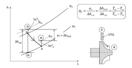
**Figure 38** Expansion process in the turbine stage [1]
