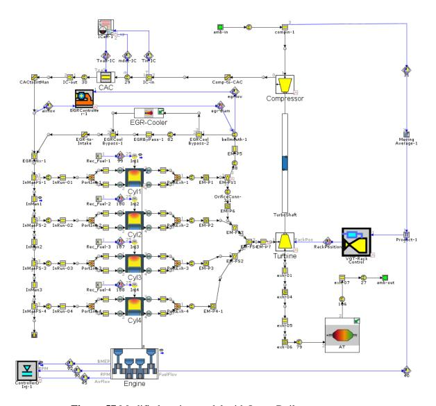
Figure 57 Modified engine model with Iveco Daily parameters
